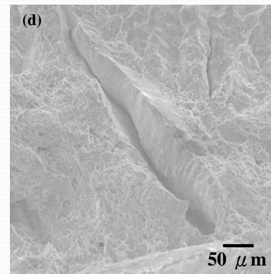
SEM micrographs showing the morphologies of the fracture surface for Alloy 182 weld after SSRT in 0.05 M HCl solution (a) at -600 mVSCE, and (c) -50 mVSCE, respectively, at a strain rate of  $8.3 \times 10^{-7} \text{ s}^{-1}$  ; (b) and (d) high magnification images for (a) and (c).
