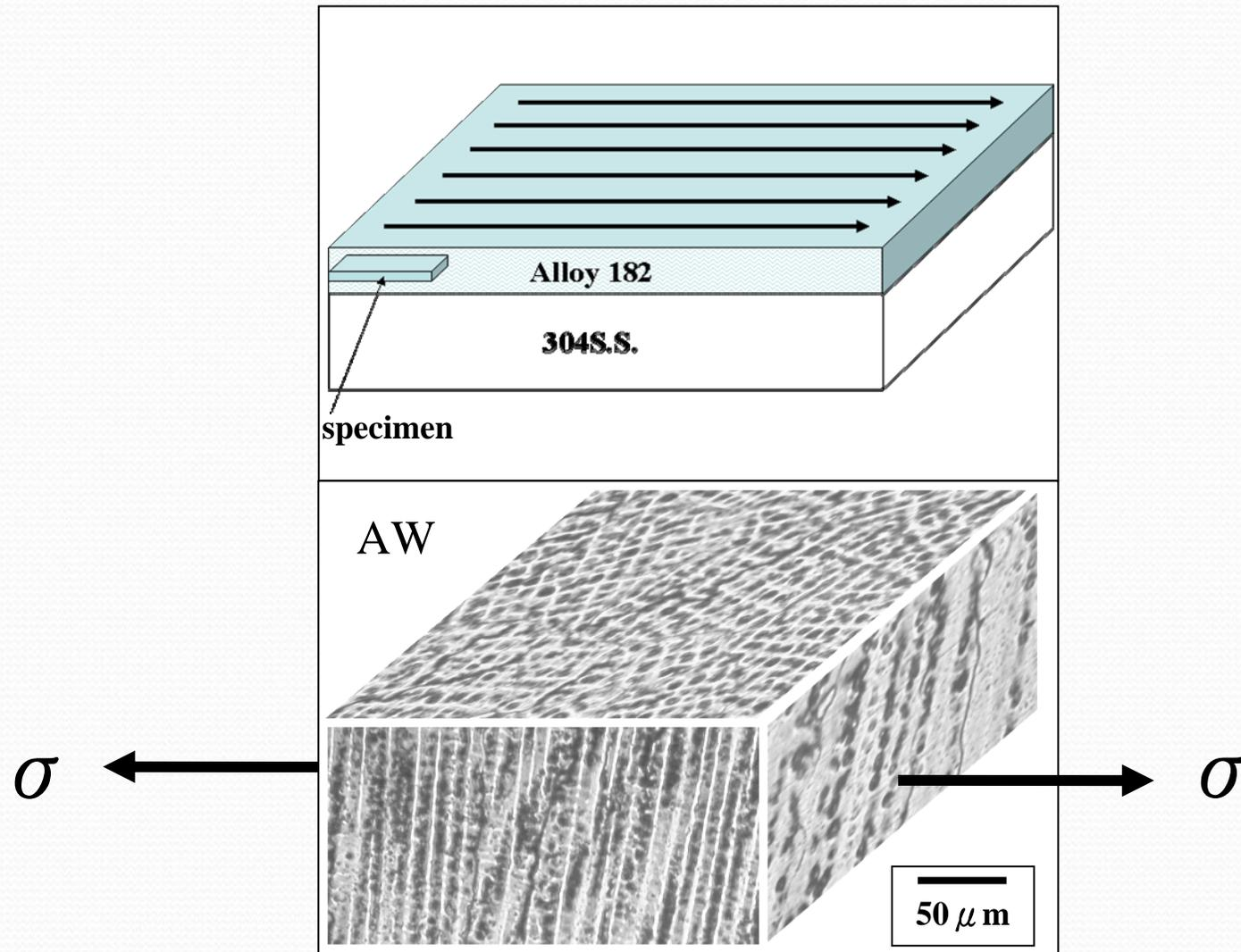
Fig. Three dimensional microstructure of Alloy 182 weld and the direction of applied stress
