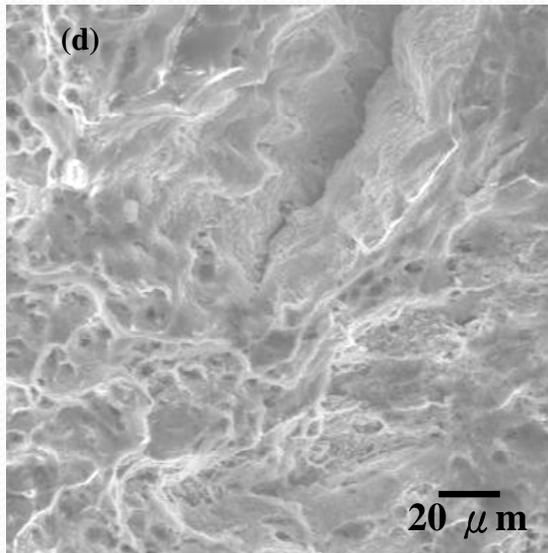
SEM micrographs showing the fracture surface morphologies for the as-welded Alloy 182 weld after SSRT in (a) air, and in 0.05 M HCl solution (c) at +60 mVSCE, respectively, at a strain rate of  $8.3 \times 10^{-7} \text{ s}^{-1}$  ; (b) and (d) high magnification images for (a) and (c).
