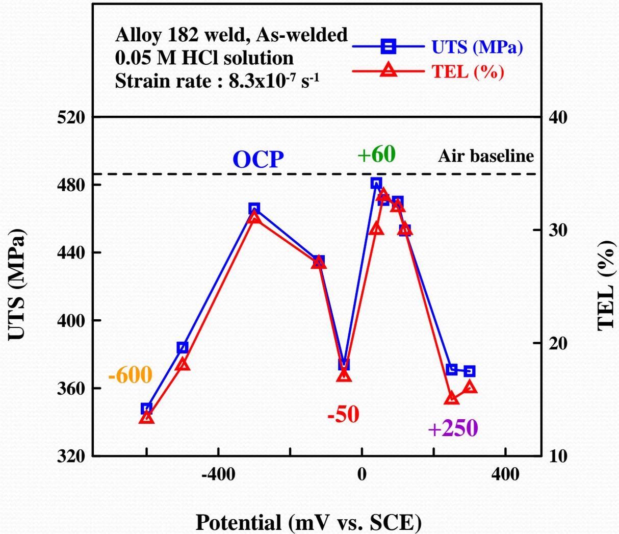
*Effect of applied potential As-welded*
